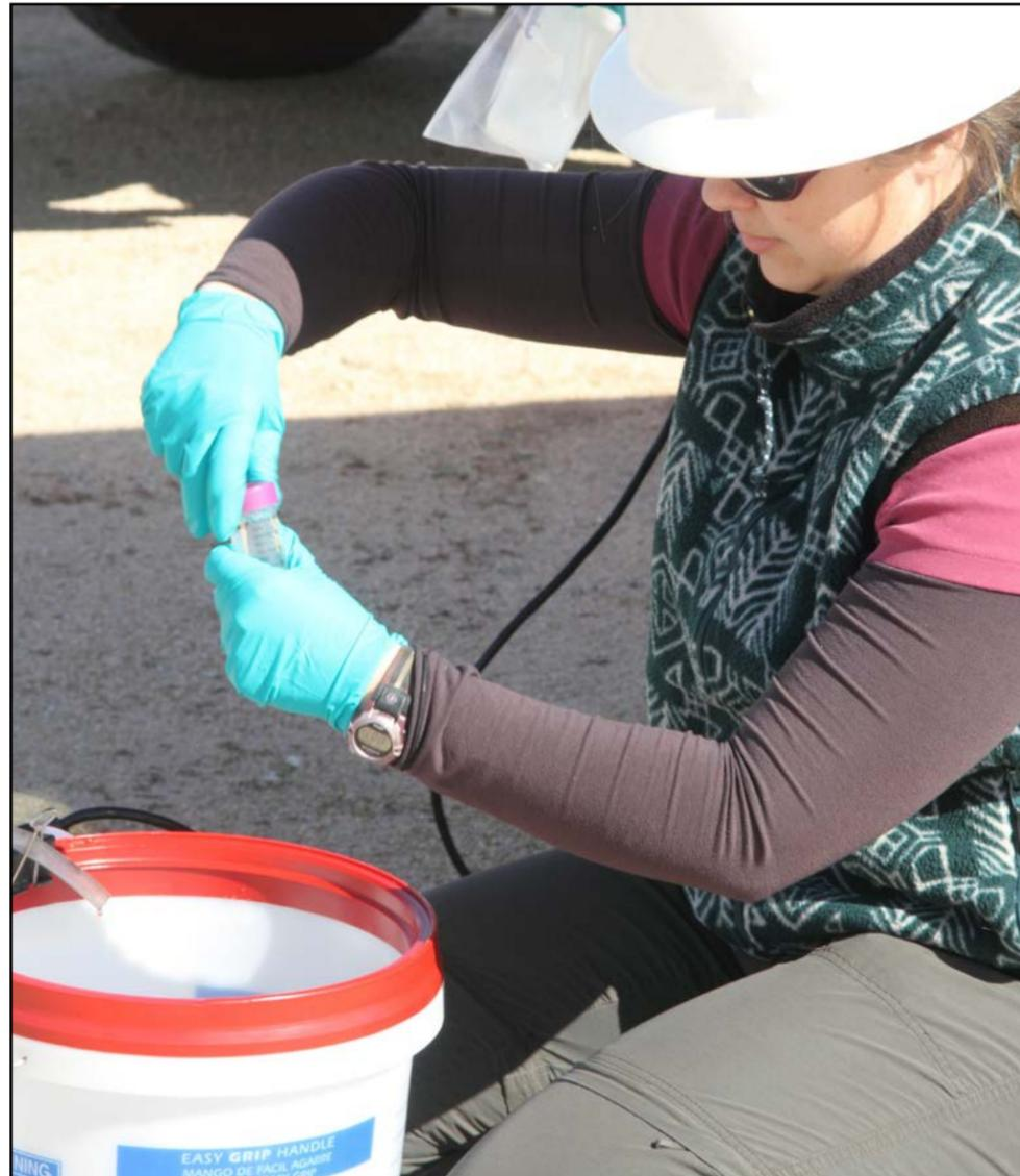
**SAMPLING GROUNDWATER:** A field worker takes a groundwater sample from a monitoring well that will be sent to a laboratory for analysis. Periodic sampling helps the Air Force track the movement of groundwater contaminants, which is evaluated during five-year reviews.
