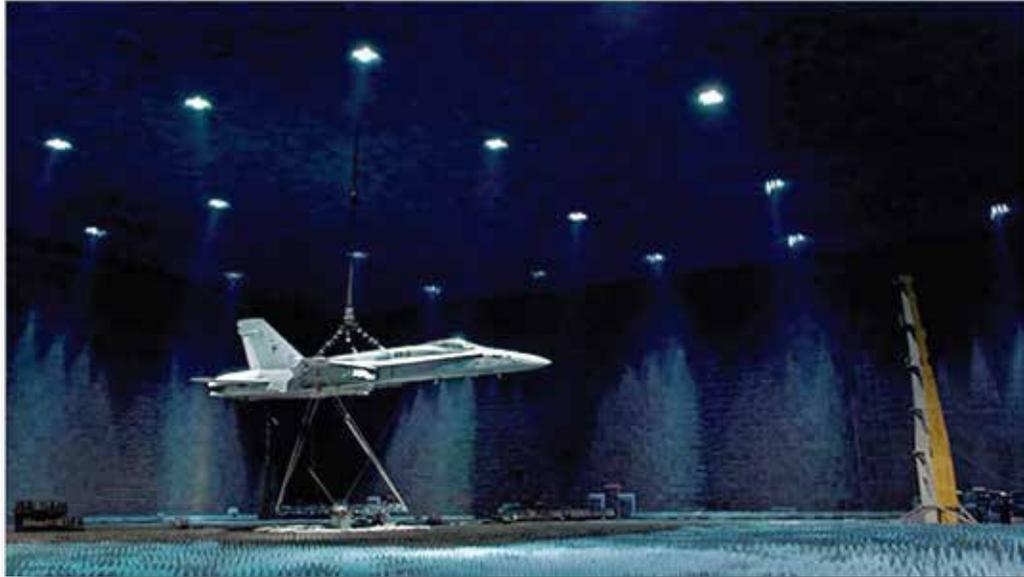
The Benefield Anechoic Facility (BAF) offers a variety of antenna pattern measurement capabilities in a particularly large indoor facility (264' x 250' x 70'). This highly flexible and secure indoor range provides extreme efficiency with uninterrupted automated test execution. This provides high throughput data collection rates.
