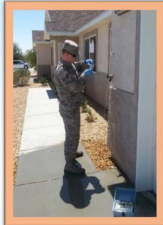
*Pictured above: Technicians from the 412th Aerospace Medicine Squadron, Bioenvironmental Engineering Flight conducting routine water testing at locations spanning the water distribution system. Water samples are collected, tested by a certified laboratory, and results are submitted to the State Water Resources Control Board to demonstrate compliance with all requirements and regulations.*
