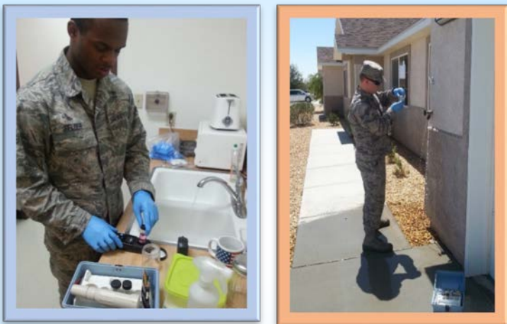
Pictured above: Technicians from the 412th Aerospace Medicine Squadron, Bioenvironmental Engineering Flight conducting routine water testing at locations spanning the water distribution system. Water samples are collected, tested by a certified laboratory, and results are submitted to the State Water Resources Control Board to demonstrate compliance with all requirements and regulations.
