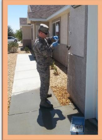
*Pictured above: Technicians from the 412th Operational Medical Readiness Squadron, Bioenvironmental Engineering Flight conducting routine water testing at locations spanning the water distribution system. Water samples are collected, tested by a certified laboratory, and results are submitted to the State Water Resources Control Board to demonstrate compliance with all requirements and regulations.*
