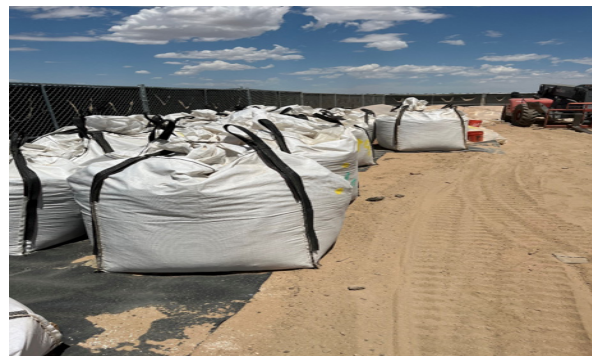
UNTREATED BATCHES —In May 2024, batches of soil contaminated with perfluoroalkyl and polyfluoroalkyl substances from three identified PFAS sites sit on the demonstration site awaiting smoldering treatment.
