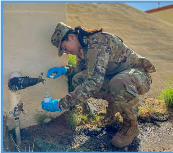
Pictured above: A technician from the 412th Operational Medical Readiness Squadron, Bioenvironmental Engineering Flight conducting routine water testing at locations spanning the water distribution system. Water samples are collected, tested by a certified laboratory, and results are submitted to the State Water Resources Control Board to demonstrate compliance with all requirements and regulations.
