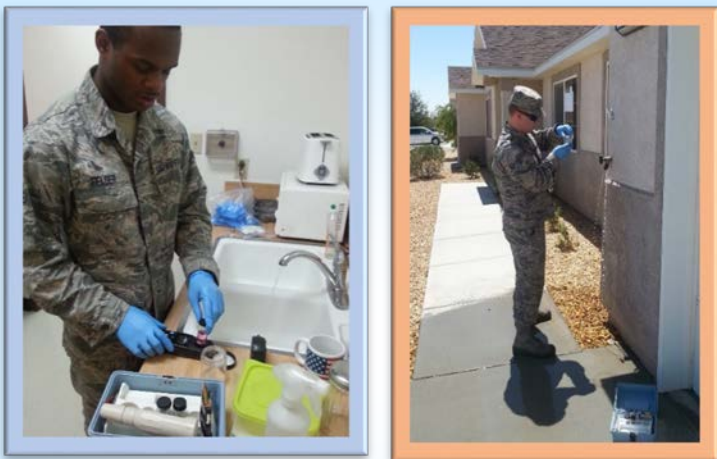
Pictured above: Technicians from the 412th Operational Medical Readiness Squadron, Bioenvironmental Engineering Flight conducting routine water testing at locations spanning the water distribution system. Water samples are collected, tested by a certified laboratory, and results are submitted to the State Water Resources Control Board to demonstrate compliance with all requirements and regulations.
