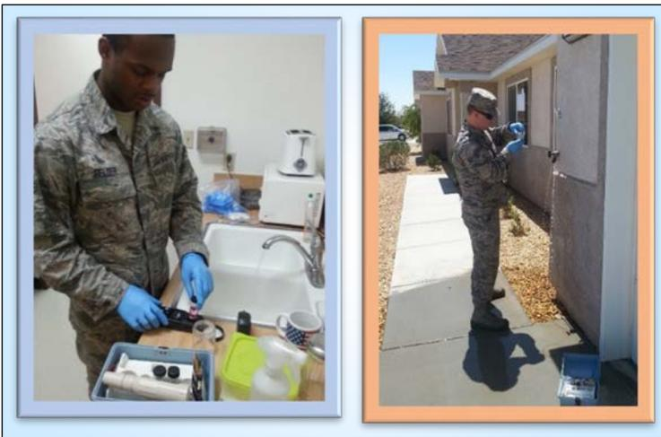
*Pictured above: Technicians from the 412th Operational Medical Readiness Squadron, Bioenvironmental Engineering Flight conducting routine water testing at locations spanning the water distribution system. Water samples are collected, tested by a certified laboratory, and results are submitted to the State Water Resources Control Board to demonstrate compliance with all requirements and regulations.*
