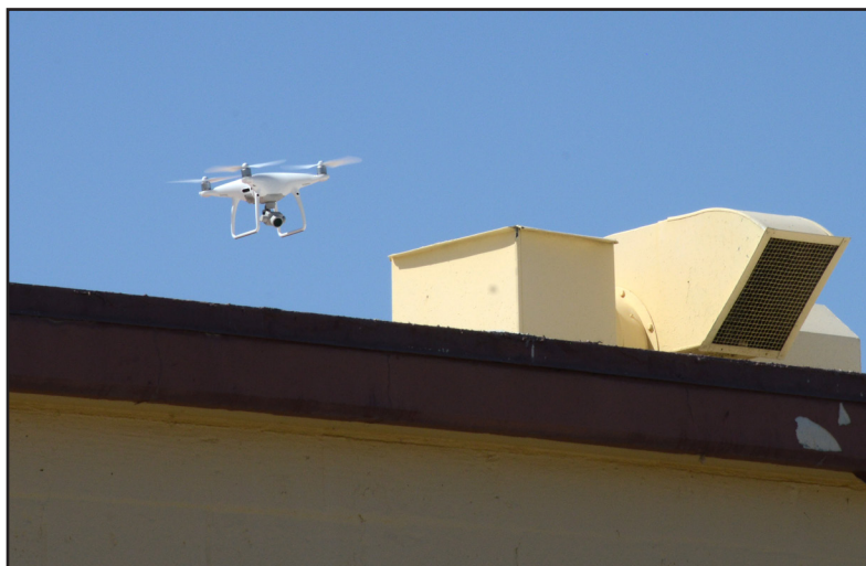
A small unmanned aerial system performs a roof inspection on Building 1401 near the Edwards flightline as part of a series of tests to determine its feasibility as an inspection tool for the 412th Civil Engineer Group. The tests were also flown to evaluate the performance of the aircraft's systems. (U.S. Air Force photo by Christopher Ball)
