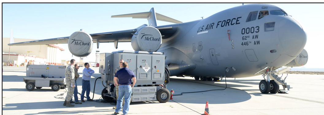
A test team monitors the Hybrid Electric Flightline Cart Technology Pathfinder unit as it powers a static C-17. The unit, which goes by the acronym HEF, was a concept demonstrator built to explore an all-electric or hybrid electrical power supply for use by flightline maintainers. Some possible advantages are lower noise, emissions and less maintenance than the diesel generators currently in use. (U.S. Air Force photo by Christopher Ball)
