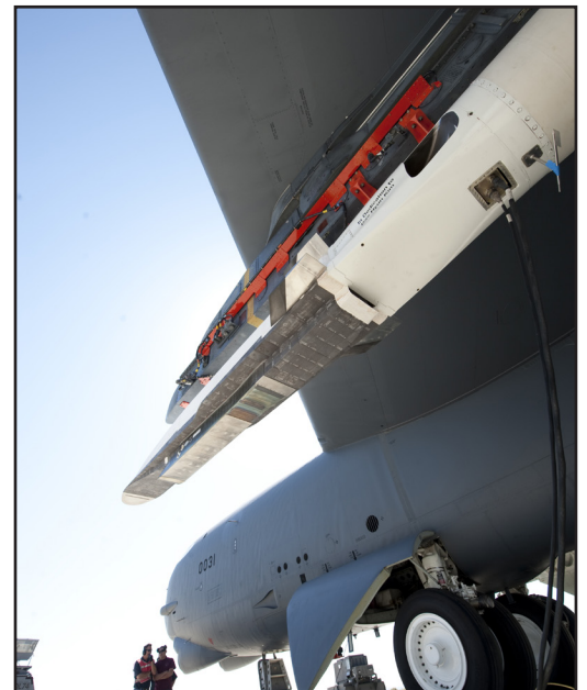
Ground crew members observe the X-51A WaveRider, which is affixed to an Edwards B-52H Stratofortress before being flown over the Pacific Ocean and launched June 13, 2011. The X-51 unmanned scramjet aircraft's maiden flight was completed on May 26, 2010. (Photo by Bob Ferguson/Boeing)
