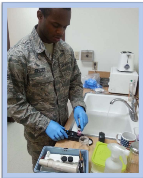
Pictured above: Technicians from the 412th Aerospace Medicine Squadron, Bioenvironmental Engineering Flight conducting routine water testing at locations spanning the water distribution system. Water samples are collected, tested by a certified laboratory, and results are submitted to the State Water Resources Control Board to demonstrate compliance with all requirements and regulations.
