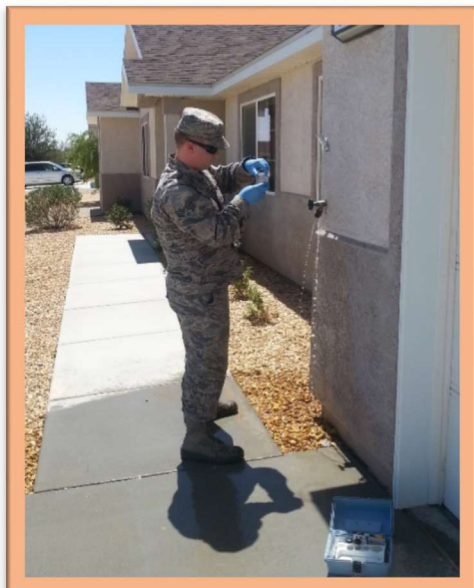
Pictured above: Technicians from the 412th Aerospace Medicine Squadron, Bioenvironmental Engineering Flight conducting routine water testing at locations spanning the water distribution system. Water samples are collected, tested by a certified laboratory, and results are submitted to the State Water Resources Control Board to demonstrate compliance with all requirements and regulations.
