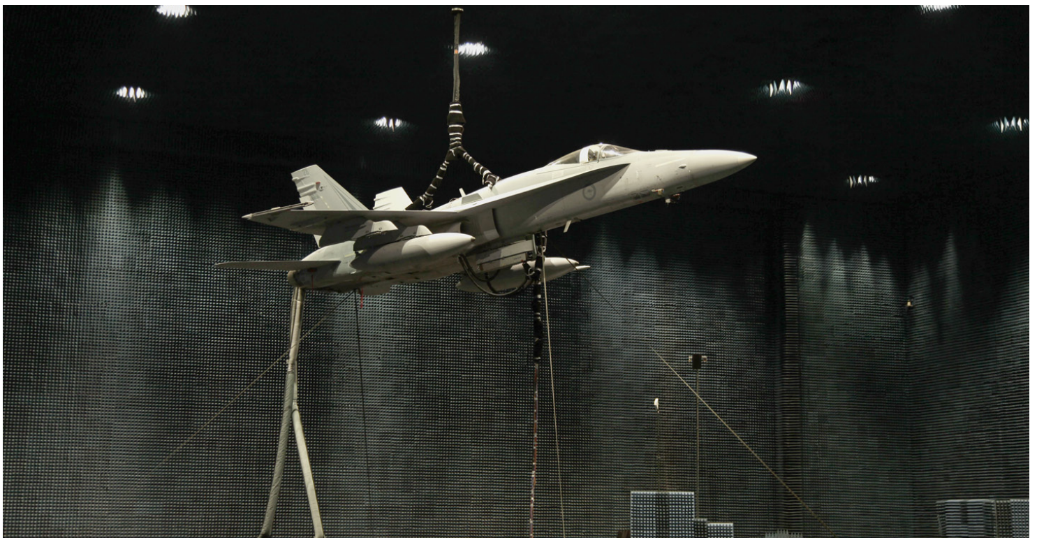
RAAF F-18 Installed Antenna Pattern Tests
